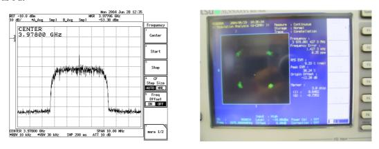
Figure 5. Measured spectrum and constellation of UWB RF transmitter
