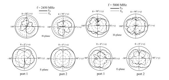
Fig. 3. Measured radiation patterns of port 1 and port 2 excitations of the proposed diversity antenna at the frequencies 2450 and 5800 MHz.
