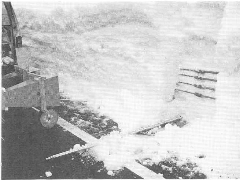
Photo 1. Four guard wires buried in snow (approximately 50 cm deep from the surface)
