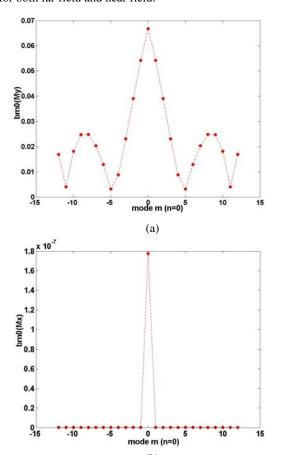
Fig.4: co-polar and cross-polar coefficients excited by an  $E_x$  -polarized normally incident wave. (a) Mode coefficient  $b_{m0}^y$ . (b) Mode coefficient  $b_m^x$
