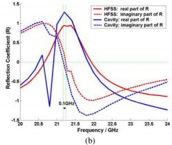
Fig.6: Real and imaginary parts of the reflection coefficient calculated using the cavity model and HFSS (based on equation (6)), (a) Lower band of square patch AMC. (b) Upper band of square patch AMC.
