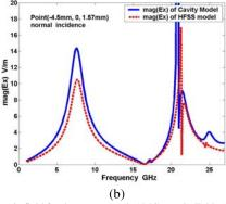
Fig.3: Electric field for the square patch AMC case in Table 1 calculated using the cavity model and HFSS. (a) Electric field at point (0,0,5.08mm) at 1GHz. (b) Electric field at point (-4.5,0,1.57mm) at 1GHz.
