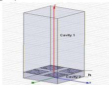
Fig. 1: Unit cell of a 2D via-less periodic structure. The shaded area is the metal patch. In this cavity model, the unit cell is divided into two cavities:
