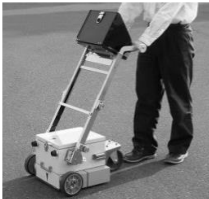
Fig. 3. Configuration of the short-chirp GPR system
