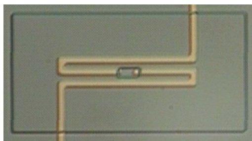
Fig. 3. Photographs of fabricated three-wire folded \lambda/2 dipole antenna.
