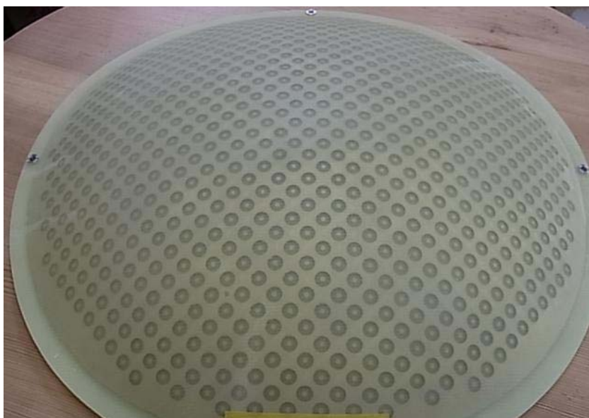
Figure 3: A photograph of the fabricated FSS-embedded radome that was used for the measurement.
