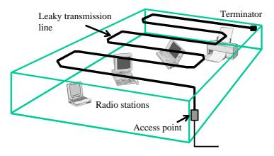
Fig. 2 System of using a leaky transmission line
