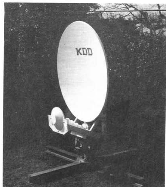
Figure 1 1.2 m Shaped offset Gregorian antenna.
