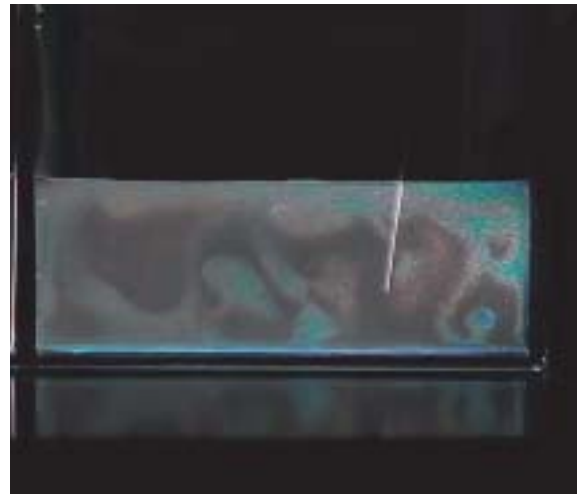
Fig. 3: Visualization of thermal convection with MTLC. Solvent is heated by the hot plate below
