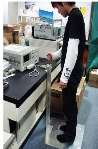
Fig.1 Measurement scenery of contact body impedance (grasping contact)
