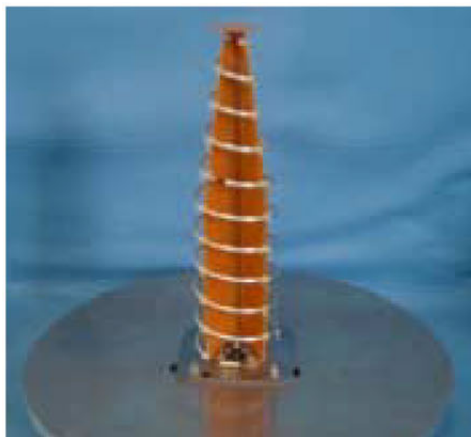
Fig.9 Photograph of LPH with conical taper-end
