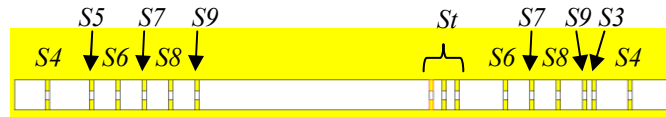
Figure 2: Switches configuration at the slot at the ground plane of the antenna
