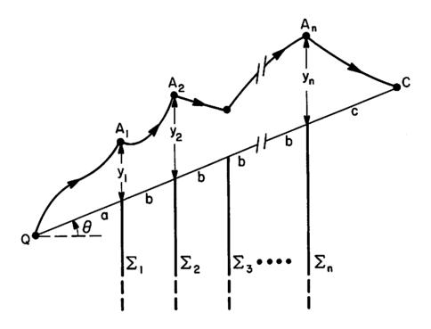
Figure 2. n equally spaced staggered half planes illuminated by the incident field from a line source at Q.
