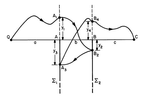
Figure 1. Two unstaggered half planes  $\Sigma_1$  and  $\Sigma_2$  illuminated by the incident field from a line source at Q.
