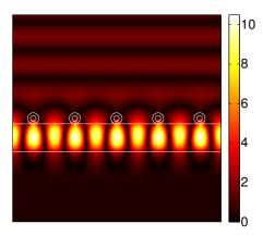
Fig. 3. Near field distribution of  $|H_z|$  for  $\lambda$ =415nm at which the guided mode resonance is observed in Fig. 2.
