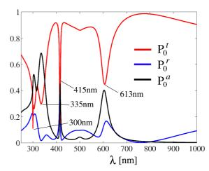
Fig. 2. Power transmission  $(P_0^t)$ , reflection  $(P_0^r)$ , and absorption  $(P_0^a)$  coefficients of the zeroth diffraction order as functions of wavelength  $\lambda$  where  $r_1$ =40nm,  $r_2$ =20nm, h=300nm,  $\varepsilon_c/\varepsilon_0$ =6.5, d=200nm,  $\varepsilon_s/\varepsilon_0$ =2.5, and the background medium is free space with  $n_B = \sqrt{\varepsilon_B/\varepsilon_0}$ =1.0.
