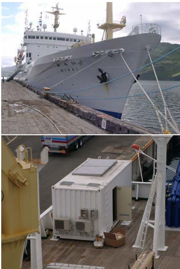
Fig.5. Japanese scientific research vessel, MIRAI, operated by Japan Agency for Marine-Earth Science and Technology (upper). On board MIRAI, developed cloud profiling FM-CW radar is settled (lower panel). Two windows on the ceiling are made of Teflon cloth.
