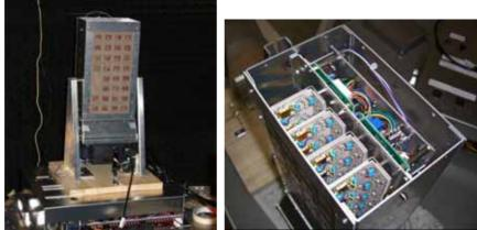
Fig. 3 Developed microwave transmitting sub-system with 32 AIAs n bent di-electric base for expand cooling area
