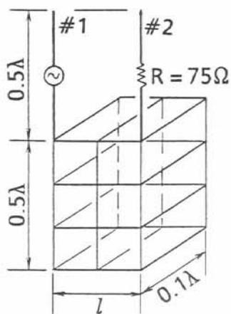
Fig. 4 Wire mesh model.
