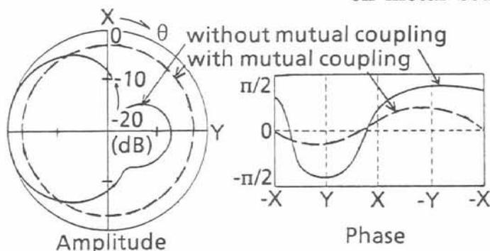
Fig. 6 Radiation patterns on metal body.
