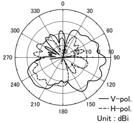
Fig.8 Elevation Pattern at 3.9GHz
