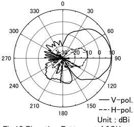
Fig.10 Elevation Pattern at 4.9GHz
