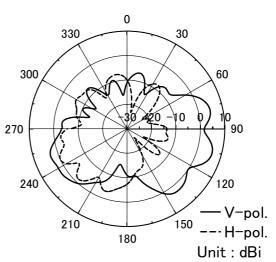
Fig.6 Elevation Pattern at 3.1GHz
