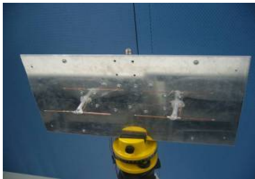
Fig. 3(a) Photo of 1x2 switched beam antenna arrays
