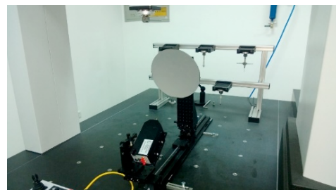
Fig.2 Sic reflector antenna under surface roughness test using three-coordinates measuring machine
