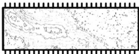
Fig. 6. H-Field surface scan just above the surface of a clock driver.
