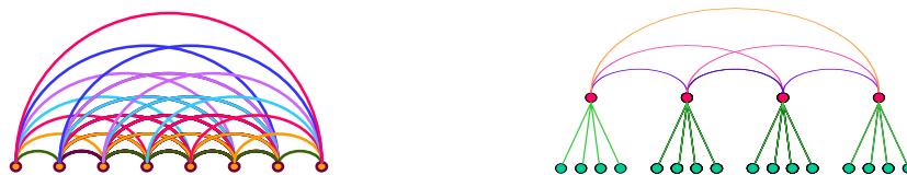
Figure 1. The analogy of a matrix-vector multiplication to a telephone network. The left picture shows a straightforward matrix-vector product, where the number of links is enormous. The right shows a two-level matrix vector product where the number of links is greatly reduced.
