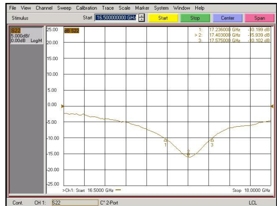
Fig. 8 the measured return loss of the proposed antenna
