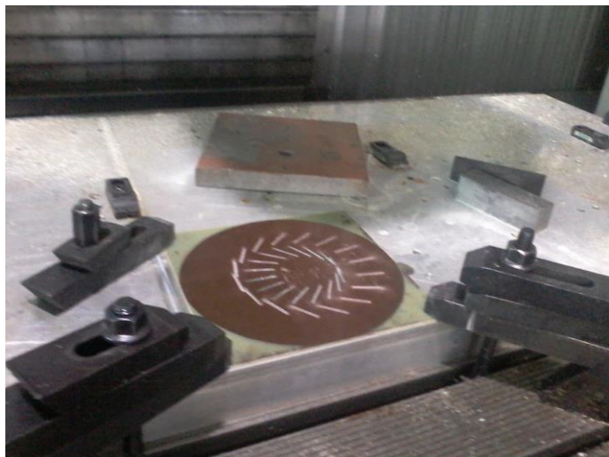
Figure 5: Slot antenna without dielectric substrate fabricated using DMF Milling Machine
