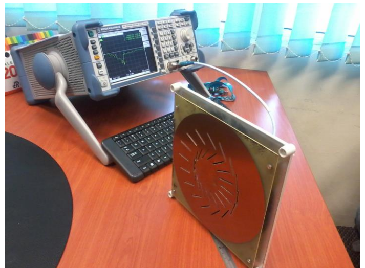
Figure 6: RLSA antenna with slot without dielectric substrate
