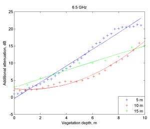
Figure 5: Additional attenuation as a function of vegetation depth at 6.5 GHz
