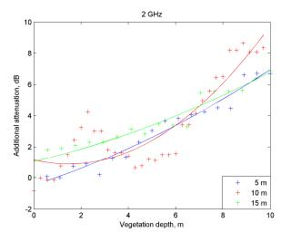
Figure 6: Additional attenuation as a function of vegetation depth at 2.0 GHz
