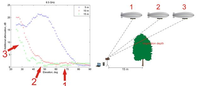
Figure 2: Additional attenuation at 6.5 GHz
