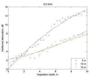
Figure 7: Additional attenuation as a function of vegetation depth at 6.5 GHz
