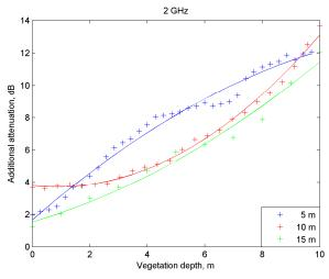
Figure 4: Additional attenuation as a function of vegetation depth at 2.0 GHz
