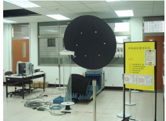
Fig.4 Compact range with impulse time domain vector network analyzer
