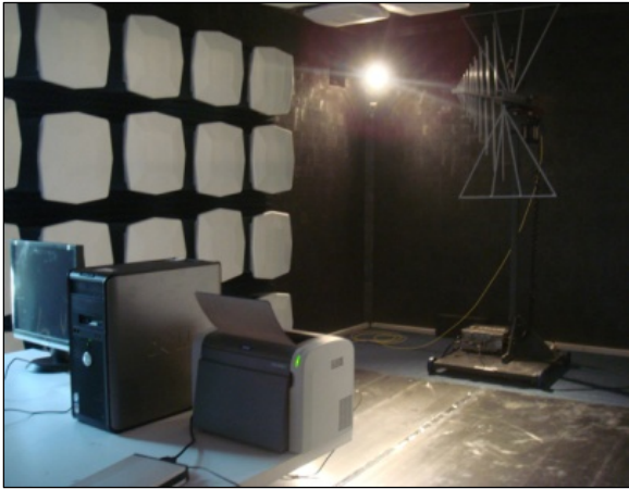
Fig.2. 7m x 4m x 3m far field range for EMI measurement
