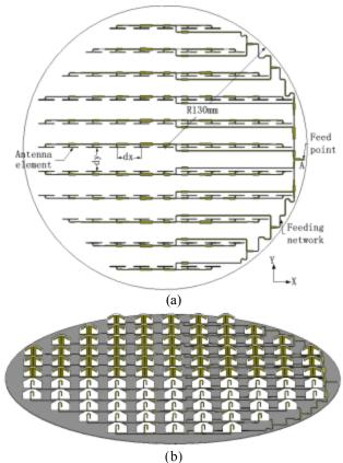
Fig.3 Configuration of the folded feeding printed dipole Array.
