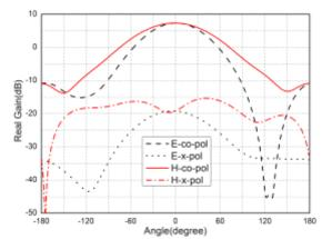
Fig.2 Radiation pattern of an antenna element.
