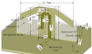
Fig. 1 Configuration of antenna element.
