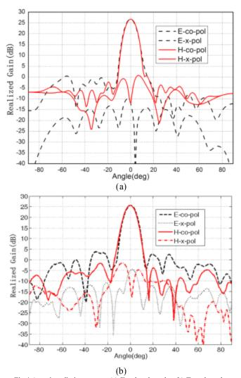
Fig.4 Array's radiation pattern. (a) Simulated results, (b) Tested results.
