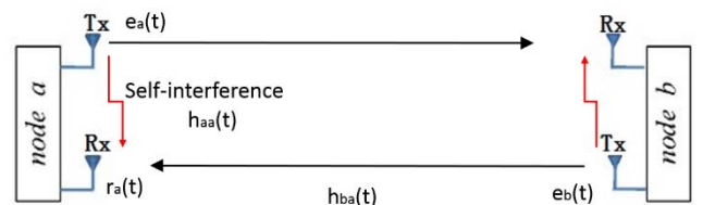
Figure 1. A simple model of full-duplex system
