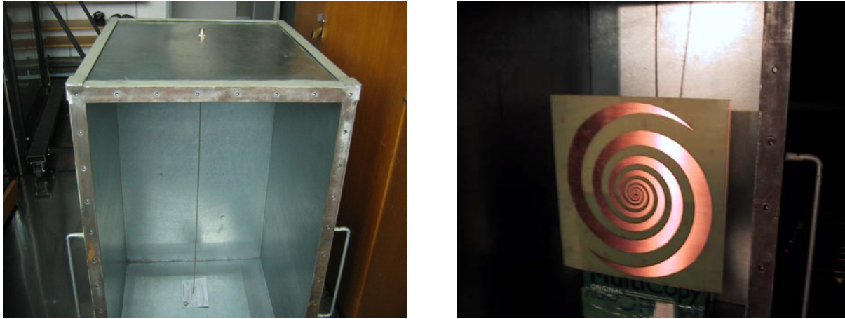
Fig. 6 Radiators – wire and spiral antenna inside the enclosure (antenna and EMC laboratory CTU in Prague)
