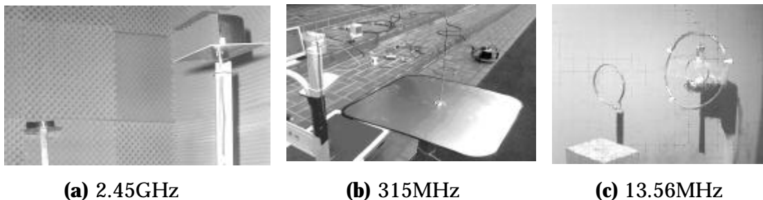
Fig.2 The appearance of the antennas for reception and transmission in access point
