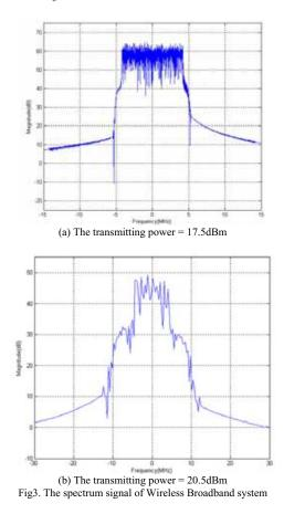
The LNA(Low Noise Amplifier) of the receiver is modeled by using 3-order polynomial model and it's coefficients are as  $a_1 = 5.01, a_3 = -3633.6$  from the data sheet of the HFA3424[8]. The output signal spectrum of Wireless Broadband system is shown at Fig3. Fig3 (a) is case with transmitting power is 17.5dBm and represent that the bandwidth is 10MHz. On the other hand, Fig3 (b) represents
