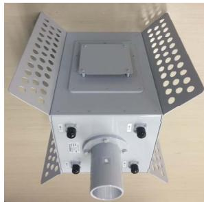
Fig. 3. Four-sector receiving antenna
