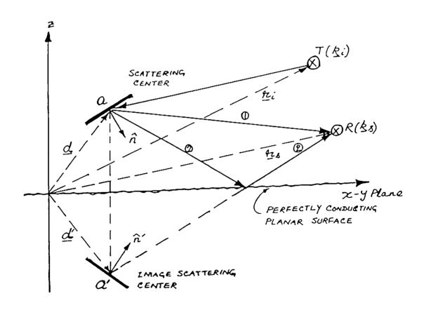
Figure 1: Geometry of the Multipath Scattering Problem
