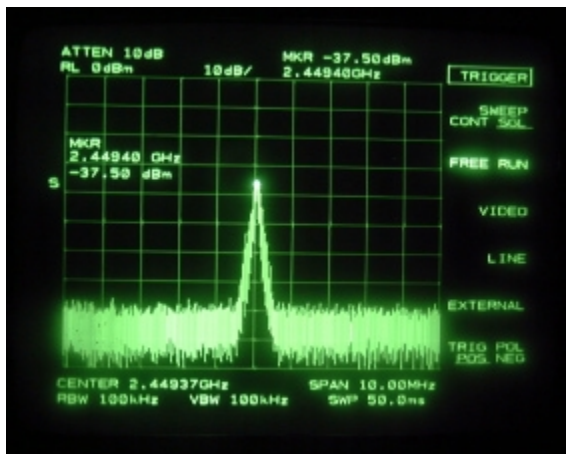
Fig. 8 The spectrum of the active integrated antenna with the oscillation layer (self-oscillating)
