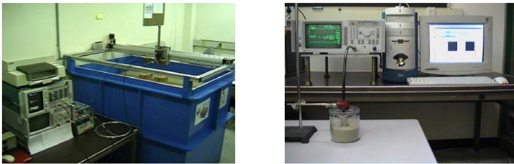
Fig. 1. Experimental setup. (a) laboratory GPR system, (b) open-ended coaxial probe system.
