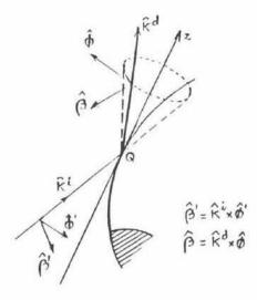
Figure 1 : Ray-fixed coordinates for edge diffraction
