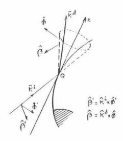
Figure 1: Ray-fixed coordinates for edge diffraction
