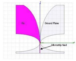
Fig. 4: Configurations of the Tapered Slot UWB antennas.
