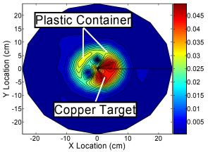
Fig. 9: Imaging Result of the 1<sup>st</sup> generation Microwave Imaging System with Calibration method A
