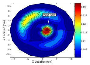
Fig. 11: Imaging Result of UWB Radar System with Calibration method B.
