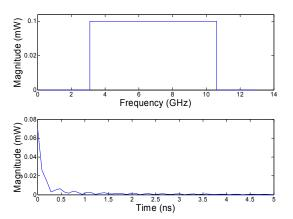
Fig. 3: Synthesized pulse (Frequency and Time Domain Representation)
