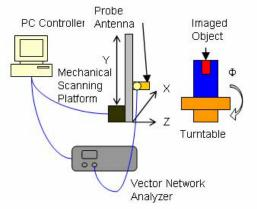
Fig. 2: Configuration of the UWB radar system.
