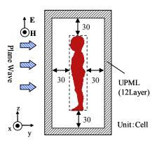
Fig. 2: Computational condition applied in this study.
