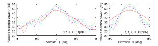
Figure 3: Simulated near field patterns.
