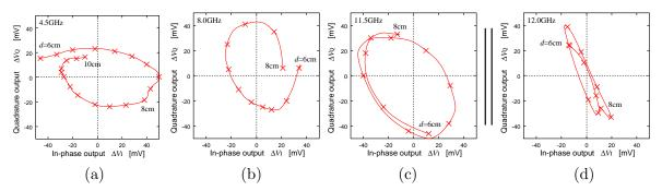
Figure 5: Homodyne output traces when a reflector is located 6cm distant from the antennas and moved with 2mm interval: (a)4.5GHz, (b)8GHz, (c)11.5GHz and (d)12GHz.
