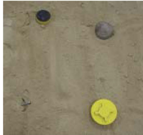
Fig. 4. Targets for the GPR experiment. On the top are the mock model of Type-72 and the stone lump. The bottoms are M8 bolt and the mock model of PMN2.
