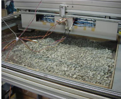
Fig. 6 An array of antennas in an inhomogeneous test site•
