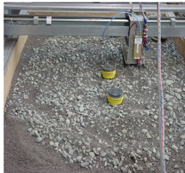
Fig. 4 TYPE 72 landmines on inhomogeneous field•
