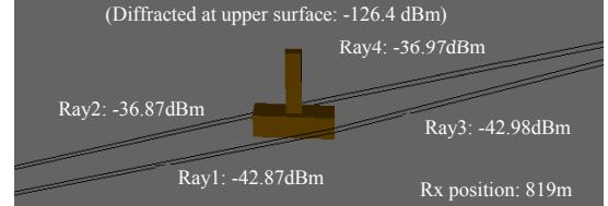
Fig. 8 Principal rays diffracted at the edge of control tower
