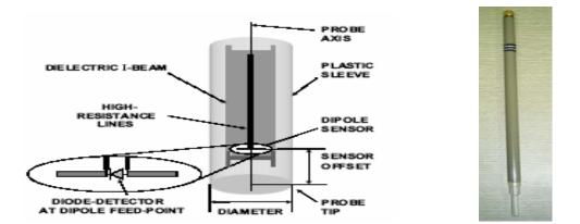
Figure 1. E-field probe features near probe tip end (left) [2] and picture of the complete probe with the plastic rod containing RF transparent transmission line (right) [3].
