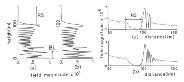
Fig. 3 Field magnitude distribution curves along the vertical observation line located at the horizontal range 95 km. The observation point P<sub>2</sub> in Fig. 1(b) is located on this line. Source height: Z'=0(m). (a) Asymptotic representation and (b) reference solution.
