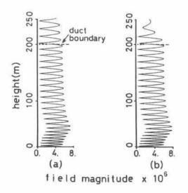
Fig. 2 Field magnitude versus height at the horizontal range 30km, with the source located 40m above the earth's surface. Observer passes through the observation points Po and P, in Fig. 1(b). Fig. 2(a) is obtained from the ray representation in Eq. (1). Two trapped rays (the direct ray (N=0, L=1) and the ray once reflected at the earth's surface(N=1, L=1)) and transmitted rays (N=0, L=1) and (N=1, L=1) are used in and above the surface duct, respectively.
