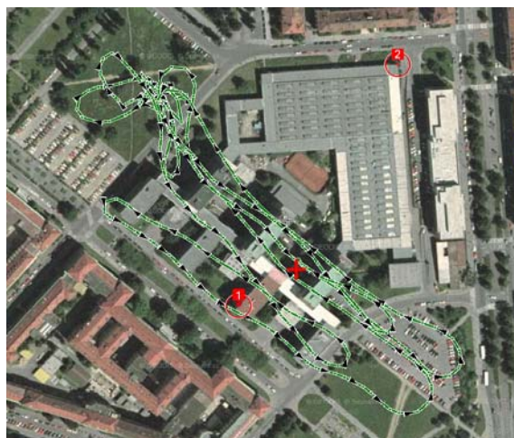
Figure 3: An Example of Airship Track during Measurement of Rooftop Diffraction
