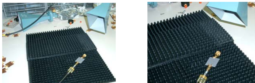
Fig. 5. Radiation measurement setup. The horn antenna is connected to port 2 of our VNA, whereas the DUT is connected to port 1, with a matched load at the output port.
