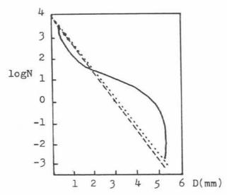
Fig.1 Rain drop size distribution (R 4.2 mm/hr).... MRT - PT ---- MP
