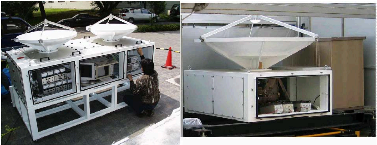
Fig.3 The developed bistatic (left) and the monostatic (right) FM-CW cloud profiling radar at 95 GHz. The diameter of the antenna is 1m for the bistatic radar and 1.4m for the monostatic radar.
